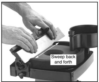
Figure 7. Grinding long knives.
